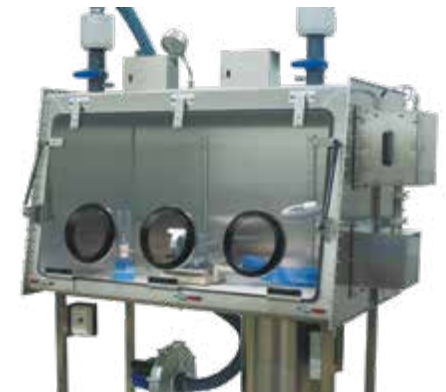
Glove box for Industry: maintenance and secured recycling of asbestos waste [aeronautics]
